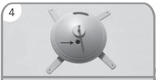
4. To fill with water, locate the cap on top of the base (A) and remove. Use a hose for easy filling. Replace cap and tighten when finished. To secure the base in ground, push L Stakes (I) through the provided holes on the legs of the base.
