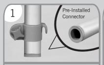
Locate the short poles (B) with the Connectors at the bottom. Add the Clamps (C) to the bottom of the poles.
