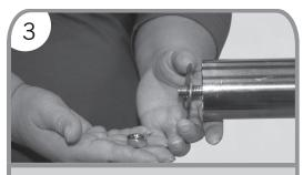
3. Unscrew the Nut (B) located at the bottom of the Post (D) and remove the Washer (C).
