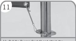
11. Pull the Bungee Cord (I) and attach the Spring Snap (K) to the Connector Plate (F) located at the bottom of the Post (D). Adjust the Tensioner (J) until the Print (L) is taut.
