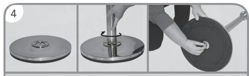
4. Take one of the Connector Plates (F) without a groove, and center on the Silver Plate (G) and Base (H). Screw the Post (D) into the hole on top of the Silver Plate (G) and Base (H). With a hand holding the Post (D), and a hand steadying the Base (H), lean the Post (D) and Base (H) on its side. Then place the Washer (C) onto the Post (D) and secure in place with the Nut (B).
