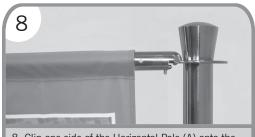
8. Clip one side of the Horizontal Pole (A) onto the Connector Plate (F) located at the top of the Post (D). Repeat for the other side of the Horizontal Pole (A) with the corresponding pole.
